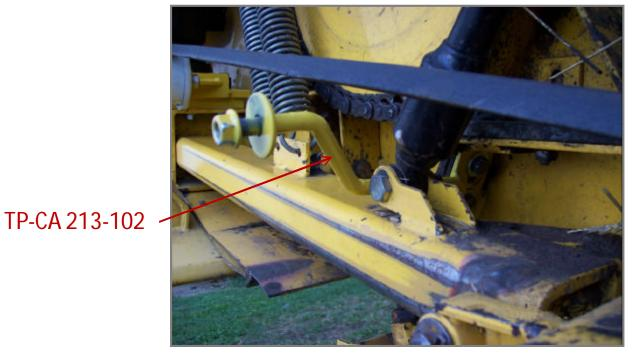
9) Once the box, basis and head blade have been positioned and they have been centered by means of fastening nuts, make the box spin and when moving it in a soft manner which will be noticed by means of the pulley, we will observe that on the other side of the platform, in its maximum movement, there will be a section out of the last finger which we recommend to cut for safety reasons so that no mobile parts remain out of the cutting bar.
